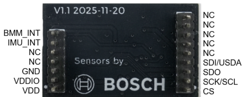
Fig. 7: ShuttleBoard-BMI270&amp;BMM350 PCB Back View (Click to enlarge)
