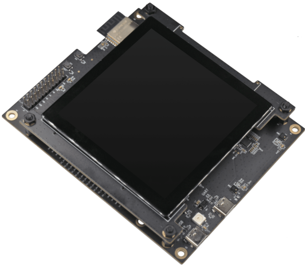
Fig. 19: ESP32-S3-LCD-EV-Board with 480x480 LCD
