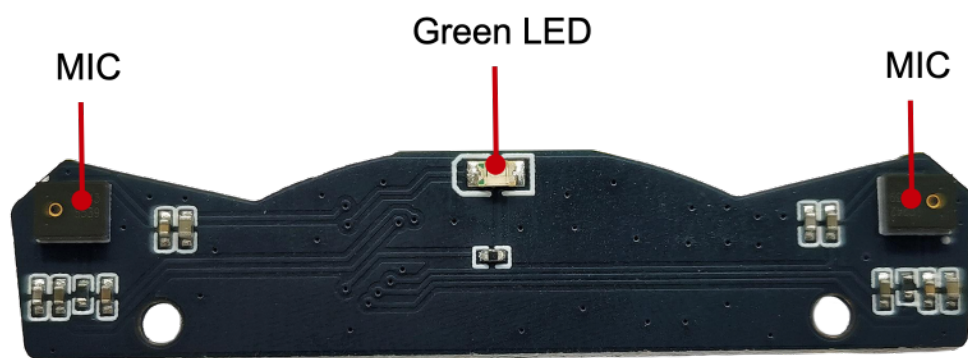
Fig. 24: ESP-VoCat MicBoard PCB Front View (Click to enlarge)
