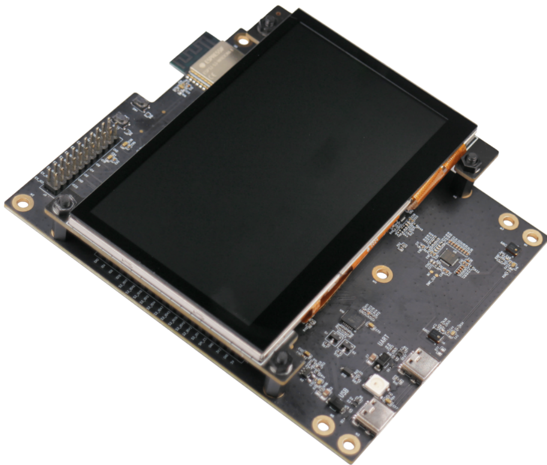
Fig. 2: ESP32-S3-LCD-EV-Board-2 with 800x480 LCD
