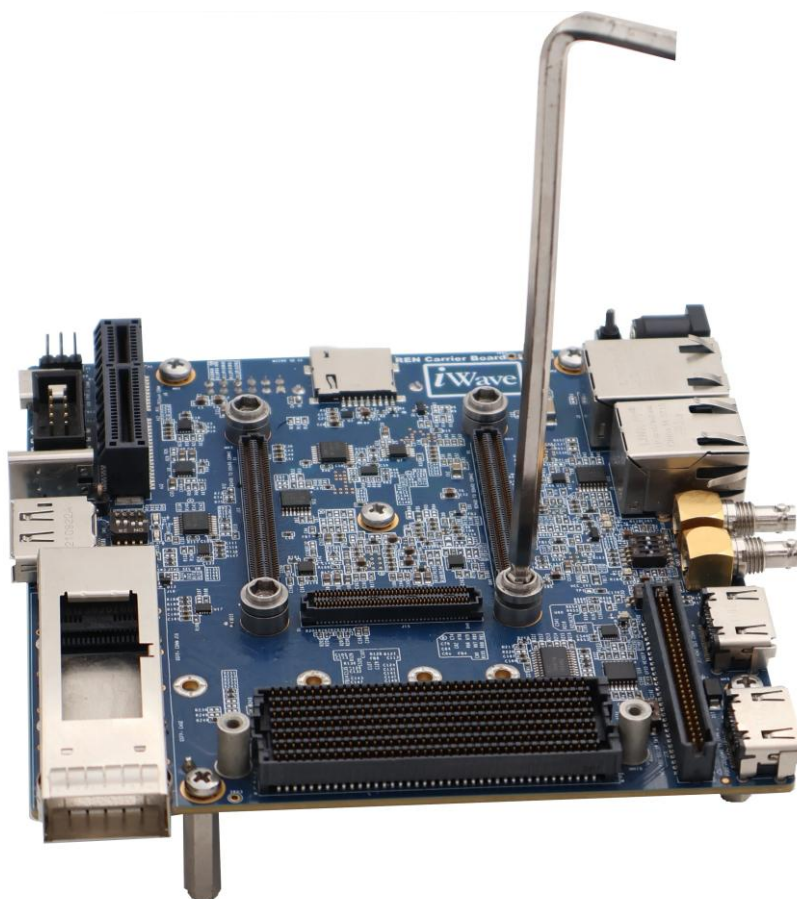
Figure 27: Tightening the of Jack Screw
