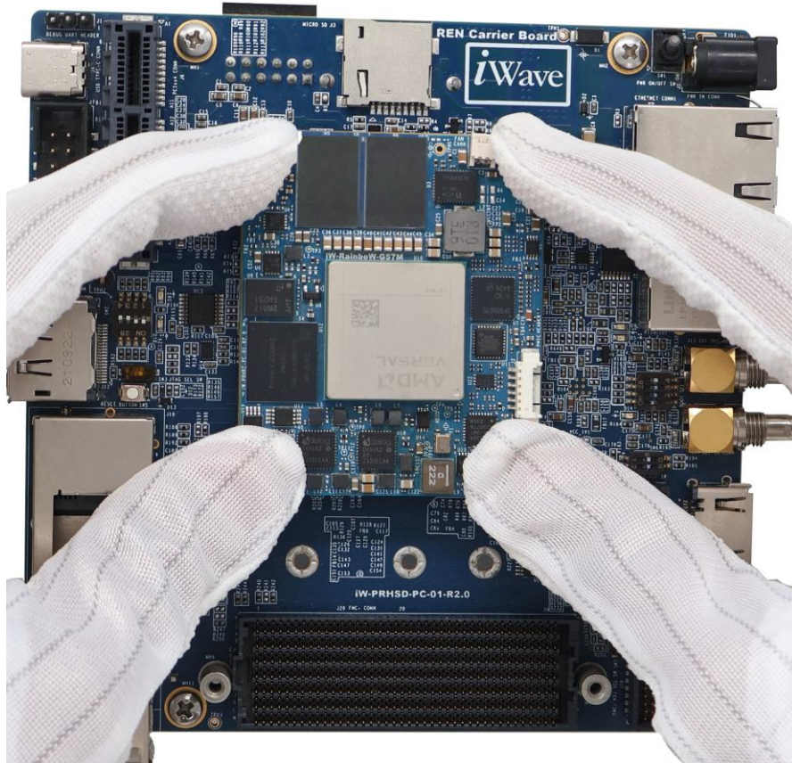
Figure 28: Insertion of SOM in to Carrier Board
