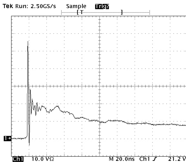
Figure 3. ESD11A5.0D Clamping Voltage Screenshot Positive 8 kV contact per IEC 61000-4-2
