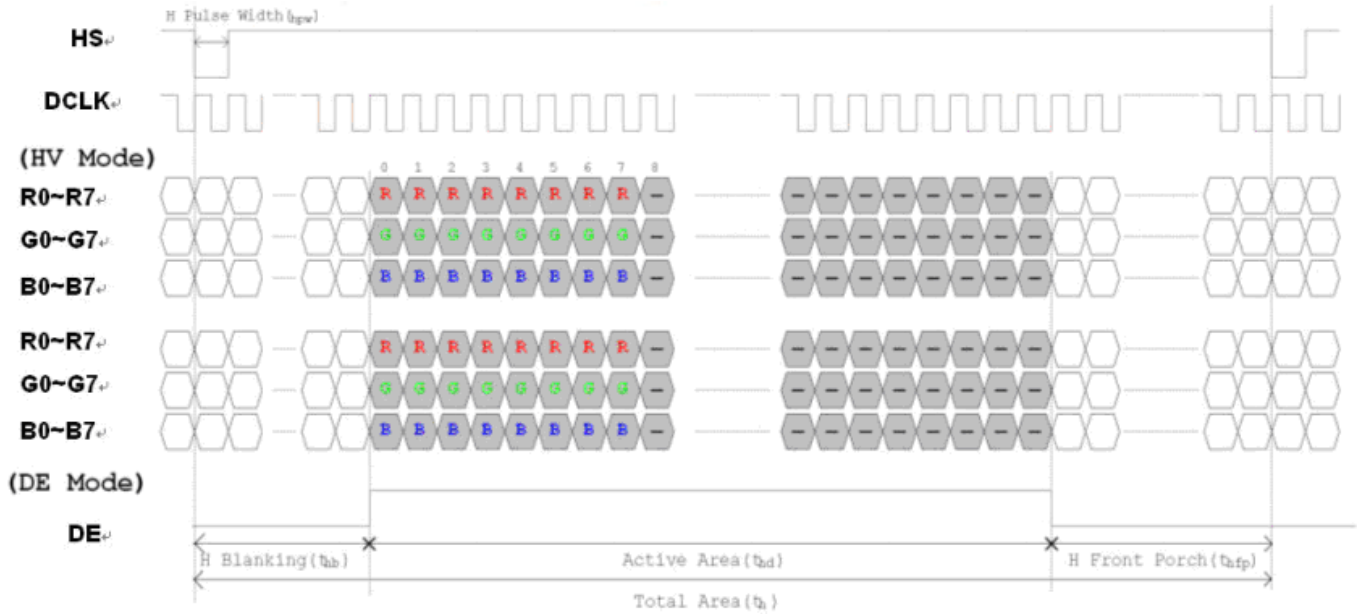
Figure 5: Horizontal Input Timing Diagram
