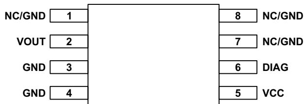
Package LE, 8-Pin eTSSOP Pinouts
