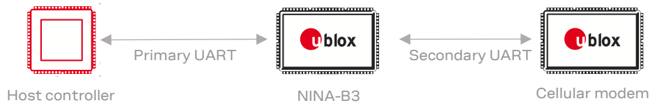
Figure 3: Example use case of the secondary UART interface
