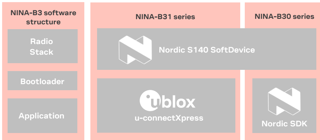
Figure 2: NINA-B3 software structure and available software options
